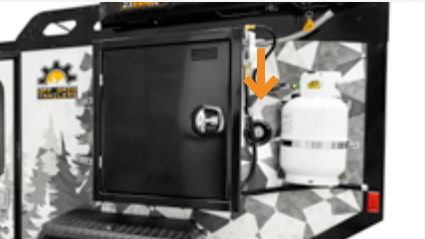
Fig 3.4 Expedition Gravity Water Fill
