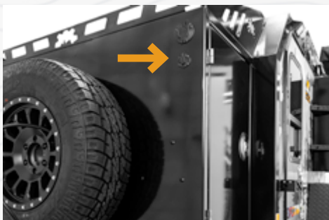
Fig 6.10 Top Plug Shore Power Lower Plug Solar Ready
