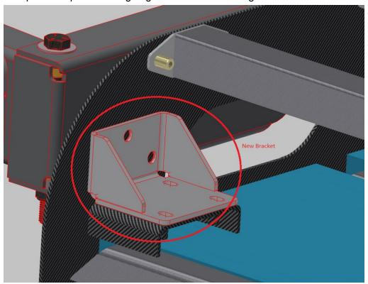
Step 2 - Attach shower assembly. Use whichever slots align with existing roof rail holes. Use locktite.
